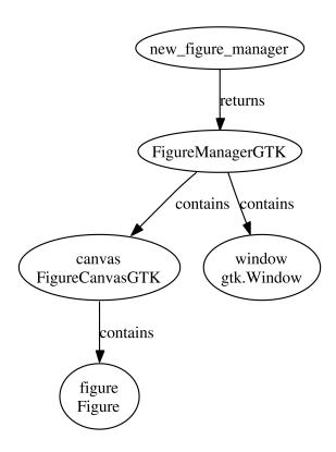
10.5: **Figure** The pylab interface function new\_figure\_manager dependent implementation returns a backend concrete of matplotlib.backend\_bases.FigureManagerBase, which contains the figure canvas and figure window. The attribute names are shown in lower case, and the backend dependent classes are shown in upper case. The standard attribute naming system allows the MATLAB<sup>TM</sup> interface to make calls across backends to the figure canvas and figure.
