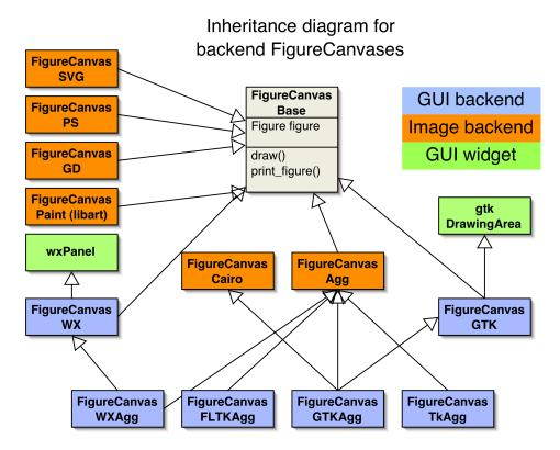
Figure 10.2: The inheritance diagram for The FigureCanvas hierarchy. The FigureCanvas is a backend dependent class which contains a figure instance. For GUI backends, the canvas should be a GUI widget embeddable in a GUI window. Some of the GUIs have backends with both native drawing and antigrain drawing (GTK/GTKAgg, WX/WX-Agg), which is readily achieved with multiple inheritance.
