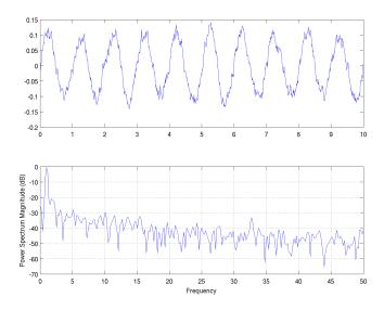
Figure 1.1: Colored noise signal and power spectrum generated with MATLAB<sup>TM</sup> as shown in Listing 1.1. Compare with matplotlib in Figure 1.2.
