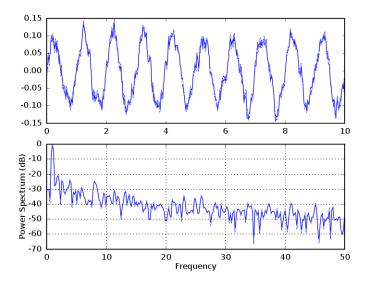
Figure 1.2: Colored noise signal and power spectrum generated with python matplotlib as shown in Listing 1.1. Compare with MATLAB<sup>TM</sup> in Figure 1.1. Note that the waveforms are not identical because they were generated from random signals!
