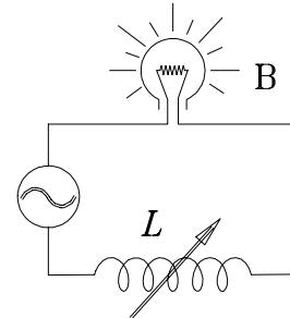
(a) What maximum inductance  $L$  is required if the power in the light bulb is to be varied by a factor of five?
