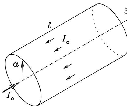
A net current  $I_0$  flows down the solid central conductor and back (in the opposite direction) along the thin outer conductor. The current density  $\vec{J}$  is uniform over the cross-sectional area of the central conductor and the returning current is uniformly distributed over the surface of the outer conducting shell.
