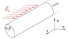
Hint: Note that this situation has cylindrical symmetry (not spherical!), with no z dependence, and hence simplifies to a 2-D plane polar problem.
