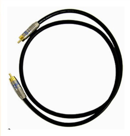
These are the “workhorse” cables used in any experiments where sharp timing signals must be transported without dispersion over distances of up to  $\sim 100$  m. They are carefully designed to have an impedance of exactly  $50 \Omega$ .
