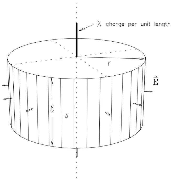
Figure 18.2 An infinite, uniform line of charge.
