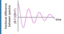
By taking the difference between the two detector signals divided by their sum, one can measure the frequency of the muons' spin precession. When different muons precess at different frequencies, the amplitude of the precession signal decays (spin relaxation). The frequency and relaxation rate tell µSR scientists about the local magnetic fields inside the sample.
