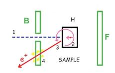
A beam of muons (1) enters the sample and stops. The muon spins precess about the local magnetic field, H (2). When a muon decays, it emits a positron (3) in the direction of its spin. This positron is detected as it goes through either the (F)orward or (B)ackward counters (4).
